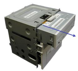
Figure 4 - 11 : Removing a 5.25-inch Device
